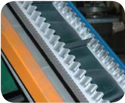
FEZ - 3.2 Industrial chemical conveyor
